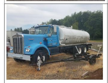
1973 Kenworth W900 Water truck. This tanker was originally purchased to haul biosolids but is now un-roadworthy. Further, the capacity of the truck is so small that no significant biosolids can be hauled. Removing the amount needed per year (700 dry tons) at the normal 3% solid would be approx. 200 loads per year. Biosolids hauling can be done more effectively by contractors. We recommend selling at public auction under Option #4.
